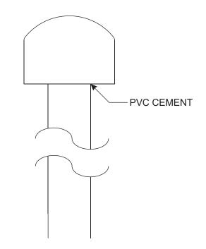
Vertical exhaust cap used with 1 1/2" PVC pipe installation. Termination cap also used with colinear transition plate model PVCT. Refer to instruction manual for venting examples.
